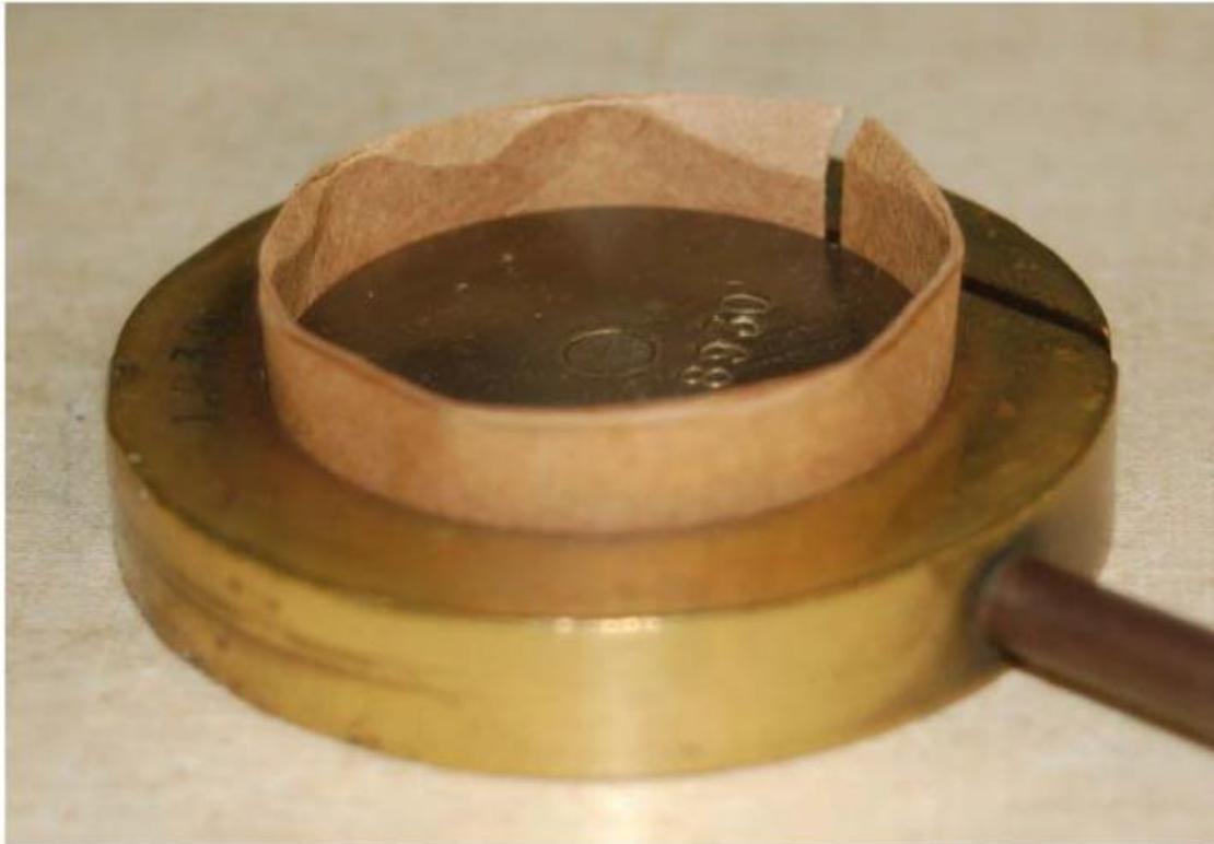
Ring Crush specimen after testing; buckling and rolling edges clearly visible
