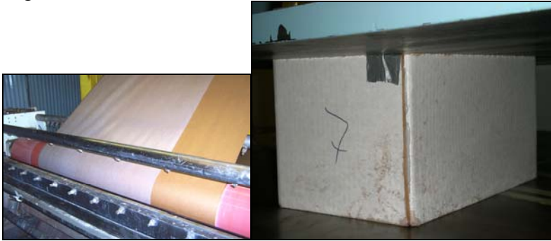
Figure 8. 42# linerboard being clay coated at Spectra-Kote left, right - a clay coated corrugated box undergoing a BCT retention test after an ice-pack 3 day test.
