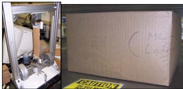
Figure 4. The IPST torsion pendulum on the left, this was written up in Appita Journal in 2008 and validates the BQM hand-held measurement of transverse shear. On the right is a BCT crushed lateral corrugated box. The lifetime of corrugated containers increases when their components are rotated 90 degrees because hygroexpansive strain is less in the MD. This data has been presented at the 2008 Progress in paper Physics Seminar in Finland.
