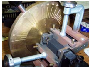
Figure 6. IPST crack angle test, a blackened sample is bent over an anvil and the angle at which cracking starts is noted.
