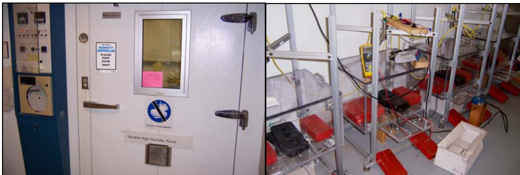
Figure 9. Left - front of the programmable humidity walk-in chamber, right - 3 of the 8 BCT creep stations inside, a post-test crushed clay coated box on floor.
