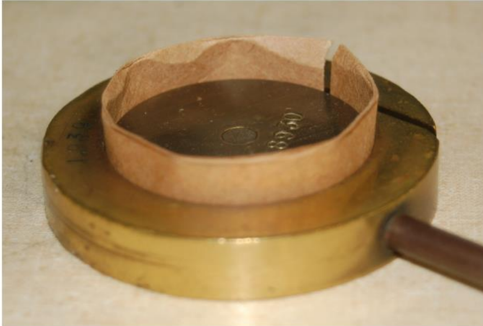
Ring Crush specimen after testing; buckling and rolling edges clearly visible
