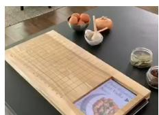
Interactive Cutting Board guides a user through meal preparation by utilizing an interactive touch screen display embedded in a cutting board. This project aims to mitigate short term memory issues associated with MCI that might affect one’s ability to cook a meal from start to finish.
