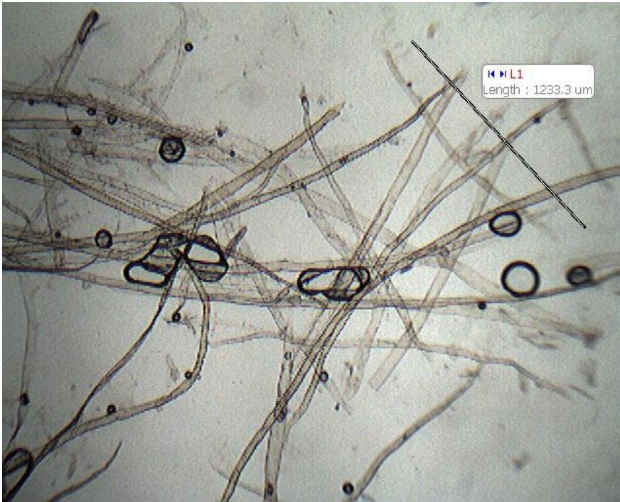
Figure 1. Stained microscopy shot 40X of virgin unbleached kraft pulp showing pine softwood fibers. This is the slide used for comparison purposes to estimate the % recycle content in other samples.
