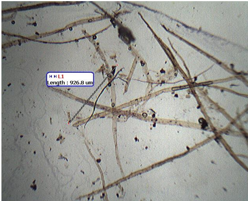
Figure 4. New World Farms box single face 40X showing the shorter gray unbleached hardwood kraft fibers among the wider longer flat softwood pine fibers. Presence of small debris fragments indicates repulping mechanical action.
