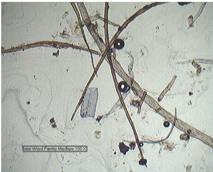
Figure 5. New World Farms medium at 100x showing bleached (gray) hardwood vessels and fibers among long flat pine unbleached softwood fibers.
